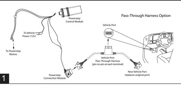
Locate OBD II Port located on underside of dash and remove two 6mm screws holding it in place.
